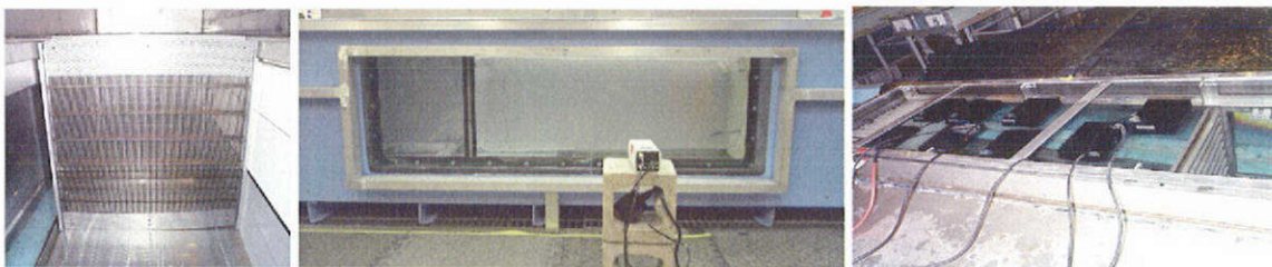
Figure 1. Bar Screen in Position, Side View of the Swim Chamber, and Infrared Illuminators Positioned Above the Viewing Window
